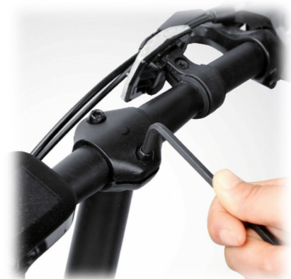
Adjustment of handlebars on electric scooter
